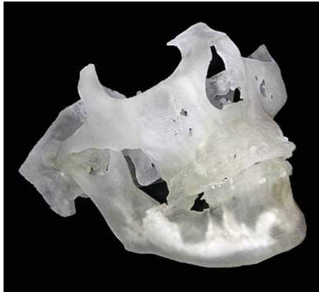
Figure C2: Physical prototype made using stereo lithography
